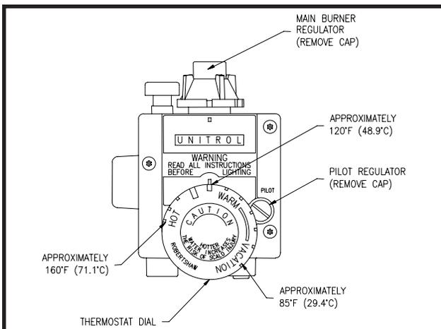
3. Change the pilot regulator by removing thermostat dial and pilot regulator cap. Depress and rotate knob clockwise to the L.P. setting using a screwdriver. Replace cap.
