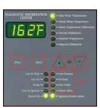
indicators prove operation and status. This monitoring system not only warns against failure, it can actually help pinpoint the source of any problems, leading to faster solutions. In addition, all of the components are field replaceable, so down-time is reduced.
