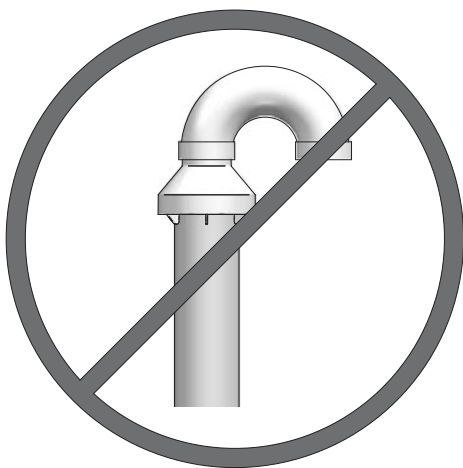
Figure 5-5 Do Not Install U-Bend to Rain Cap
