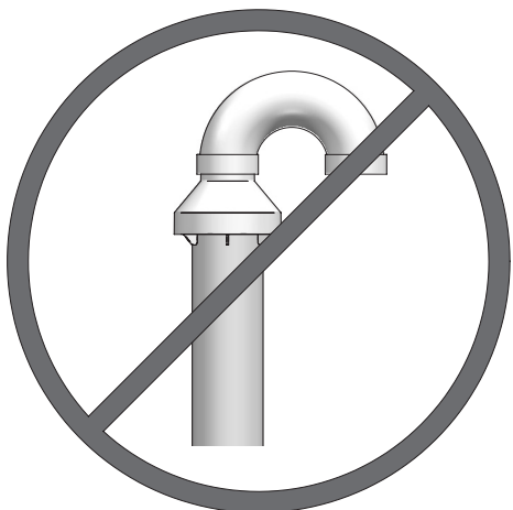
Figure 5-5 Do Not Install U-Bend to Rain Cap
