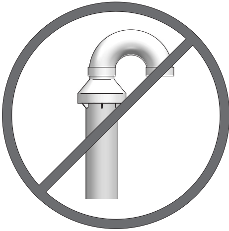
Figure 5-5 Do Not Install U-Bend to Rain Cap
