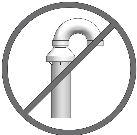
Figure 5-5 Do Not Install U-Bend to Rain Cap
