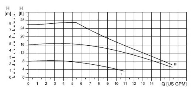
PWM or 0-10 VDC input control is also available for this pump.
