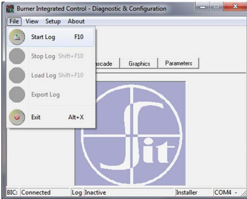
By clicking **File** to access the drop down menu (FIG. 4-1), all logging functions are now accessible. Click **Start Log** or **F10** to select a Save As location and File Name for the WinPro log file. If logging for a short period of time, click **Stop Log** or **Shift+F10** when all of the desired data is acquired. This will complete and save the log file.
