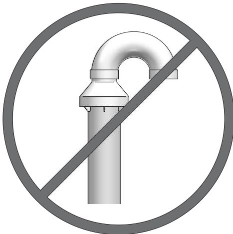
Figure 5-5 Do Not Install U-Bent to Rain Cap
